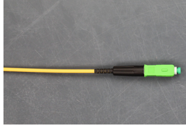
Step 18: Screw the tail boot up all the way to complete the assembly.
